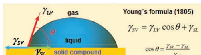
Fig. 7 Calculation of the contact angle of the freely lying drop of the tested liquid
