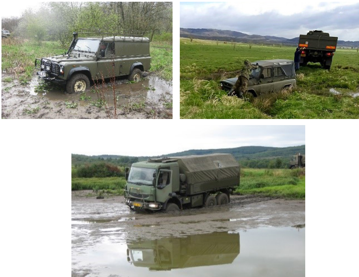
Fig. 1. Examples of wrong evaluated trafficability of terrain.
