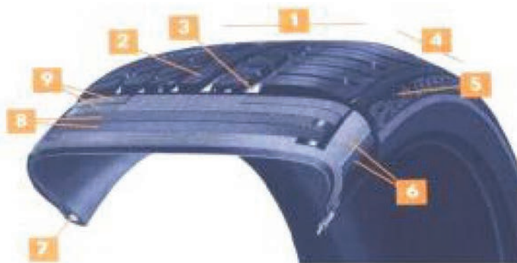
Fig. 2 Passenger tire construction. Explanations to the Fig. 2.: tread (1), positive sample (2), negative sample - groove (3), tire arm (4), sidewall (5), tire carcass and tire bead (6), heel rope (7), bumper (8), PA bumper and flag (9) [4]
