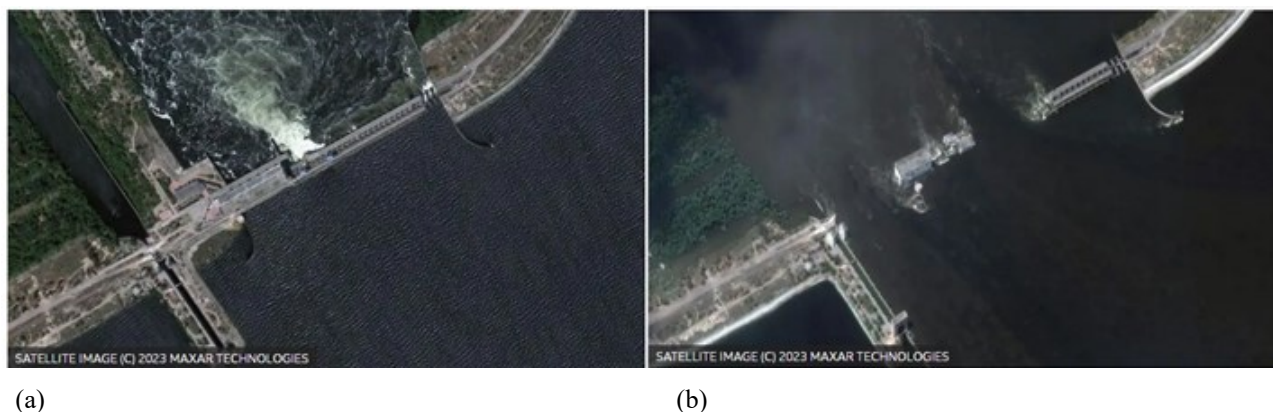
Fig. 1 Kakhovskaya HPP on June 5, 2023, the day before the dam breach: (a) (left) and (b) Kakhovskaya HPP a day after the dam breach, on June 7, 2023 (right). Source: https://www.bbc.com
