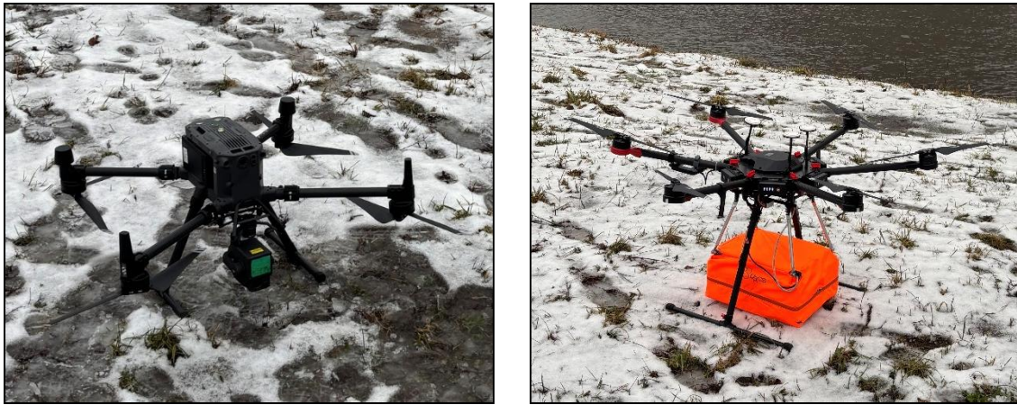
Fig. 1. Unmanned platforms used in the measurements – (A) LiDAR system; (B) ground-penetrating radar system
