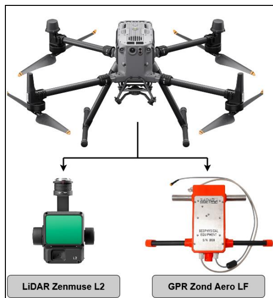
Fig. 7. Conceptual design of a modular unmanned aerial vehicle for engineer reconnaissance of a water obstacle
