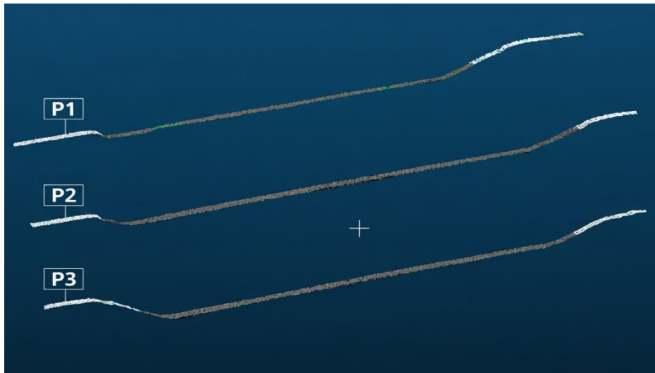
Fig. 5. DMR 5G digital terrain model with an indicative determination of the watercourse width
