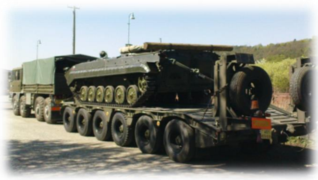
Fig. 2 Tatra T-815 8x8 with P-50 N low-loader transporting tracked vehicles
