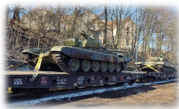
Fig. 3 T-72 tank secured on an Smmps 54 railway flatcar [OSINT defender]
