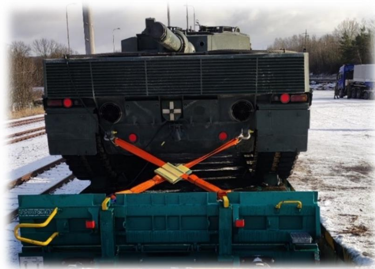
Fig. 4 Securing the Leopard 2A4 tank to a Sammns-X railway flatcar
