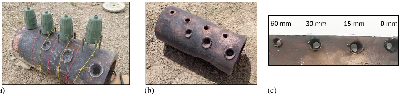
Figure 2. Overall result of the previous experiment with 3D-printed copper-filled liners: (a) arrangement of the shaped charges with 3D-printed liners on the steel target before detonation; (b) steel target after detonation, showing the four rear entrance holes corresponding to the lined charge configuration; (c) outlet holes on the inner side of the steel cylinder corresponding to the tested stand-off distances.
