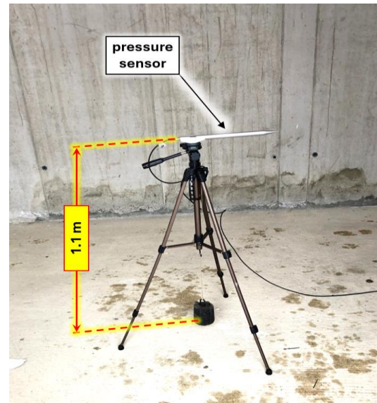
Fig. 2 Pressure sensor mounted on tripod at 1.1 m above the floor
