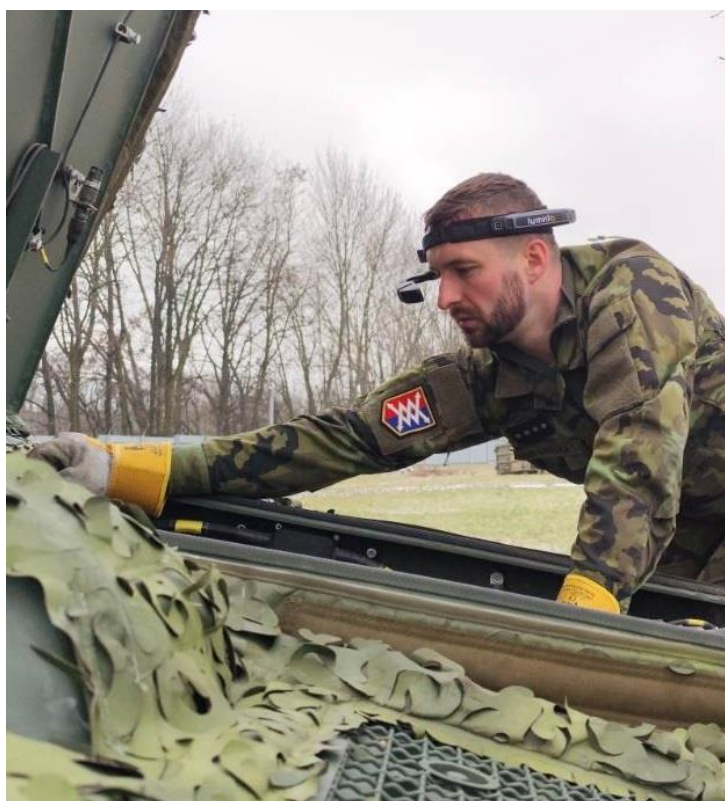
Fig. 1 The image captures a field diagnostic activity during the inspection of technical equipment, in which a modern hands-free diagnostic device with assisted-reality capabilities and support for remote collaboration is used.
