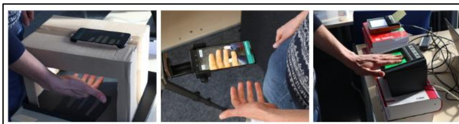
Fig. 7. Example of scanning setups using various scanners (from left: contactless "box" scanner, phone on a tripod, touchscreen scanner) [7].
