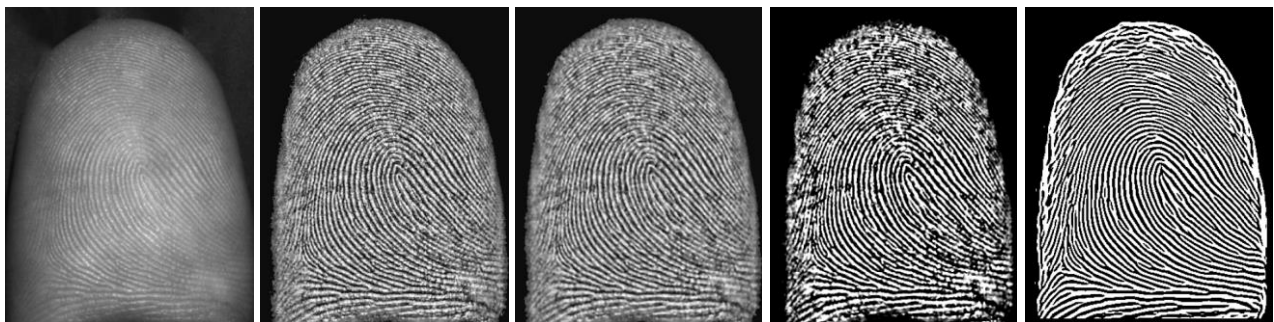
Fig. 9. Examples of the fingerprints (from left): original; CLAHE; median filter; normalized; final [9].
