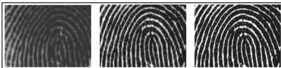
Fig. 2. Comparison of images with different resolutions (left: 380 DPI, center: 500 DPI, right: 1,000 DPI) [5].
