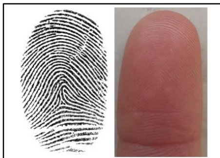
Fig. 3. On the left is an image from a touchscreen; on the right is a photo from a cell phone [7].
