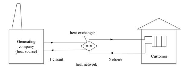
Fig. 7. Schematic circuit of an independent heat supply system
