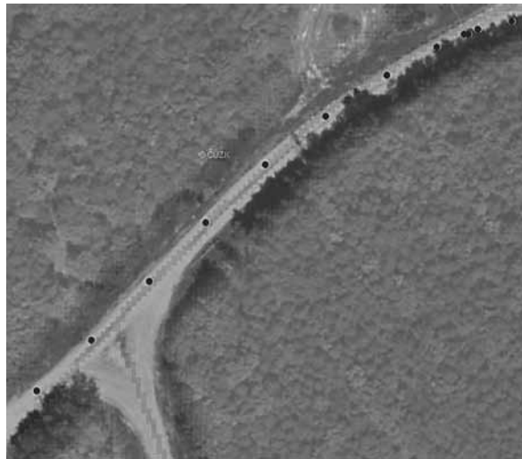
Figure 9. Superposition of the cost map (gray scale), measured vehicle position (PANDUR II, red dots), and orthogonalised aerial image
