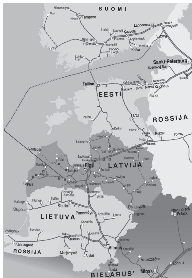
Fig. 3. Baltic gas supply grid
